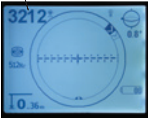
Tracing sondes: when this number increases you approach the target
