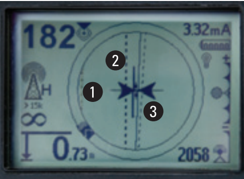
Screen in Omniseek mode: See multiple lines (Screenshot shows three different lines) ①, ②, ③
